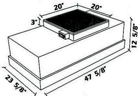
**Housing:** White powdercoated, fabricated from 20 gauge steel, joined and positively sealed with a gasket to HEPA filter.
